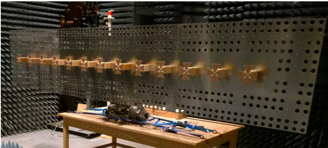
Figure 2-3: FFI produced and NTNU/FFI designed 11 element dual-polarised antenna based on dual-bowtie elements. One terminated element at each end is added to avoid large differences in the antenna pattern and mutual coupling of the connected elements.
